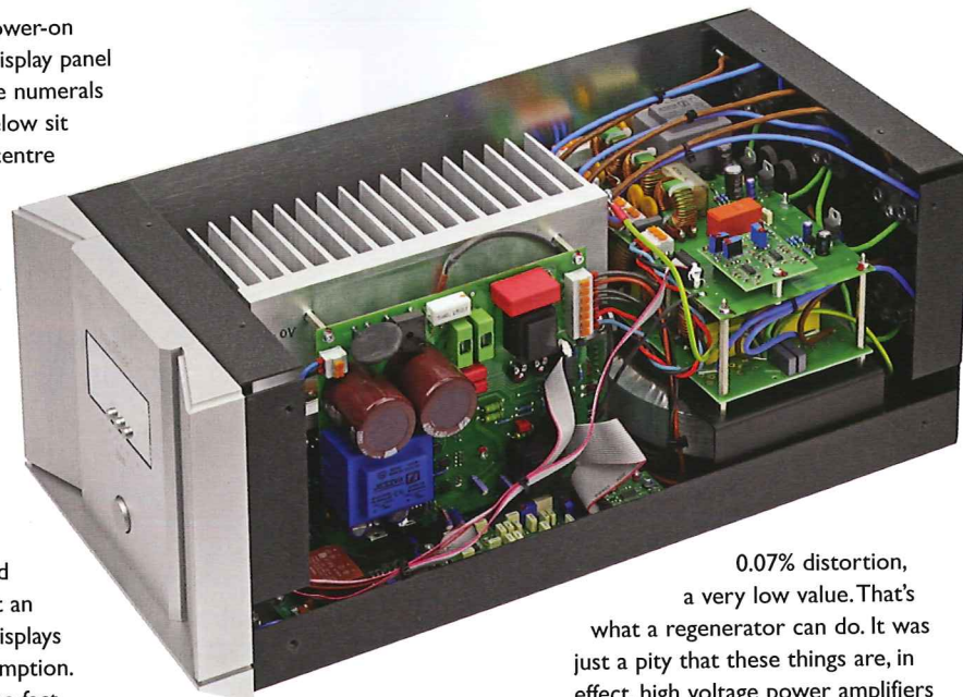
A complex interior with large heatsink of the 150 Watt high voltage amplifier dominating.
