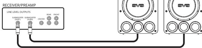
If you have more subwoofers than Sub Outputs from your AV Receiver, an easy solution is to use an RCA splitter or RCA Y-adapter to divide the subwoofer output. This is the most commonly recommended way to connect multiple subwoofers when there is only one Sub Out.
