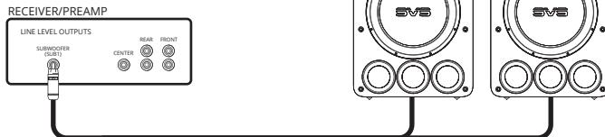
Another option is to use the Left and Right RCA or XLR outputs on the PB17-Ultra R|Evolution to Daisy Chain additional subwoofers. It's important to use the matching output and input terminals. For example, if you are using the RCA inputs, be sure to use the RCA outputs to daisy chain to the next subwoofer.
